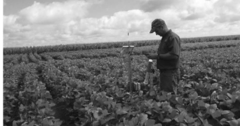
Fig. 3. Another type of sensor actually measures the canopy temperature. When the canopy gets a certain set temperature (different for various crops) for a number of hours and IRRIGATE ! signal is sent.
