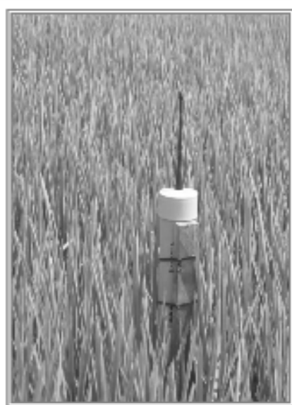
Fig. 2. Another type of sensor transmitter peaking over the canopy of rice grown under a pivot. This device handles three moisture sensors and one temperature sensor. Problems in communication can occur if the transmitter is not higher than the canopy, which was happening here.
