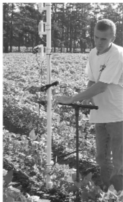
Fig. 1. A mounting pole secured in place inside a buried PVC pipe for easy breakdown to allow equipment to pass. Sensors are buried and hooked to transmitters mounted on the pole which forward data on to a desktop computer.
